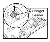
Set the charger cleaner onto the transfer charger and gently slide the cleaner in the direction indicated by the arrow two or three times.
